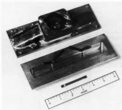
Fig. I-12 Window target. The filled and sealed tube in the foreground is held in the slotted window area by the bronze clamps.
